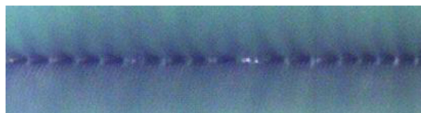
Figure 13. Irregular coating streaks captured by high speed camera. Large molecular weight (approximately 1,000,000 molecular weight) polymer (super yellow: commercially available yellow light-emitting polymer) causes extensional viscous flow between the gravure roll and substrate, which creates unwanted streak patterns of polymer.
